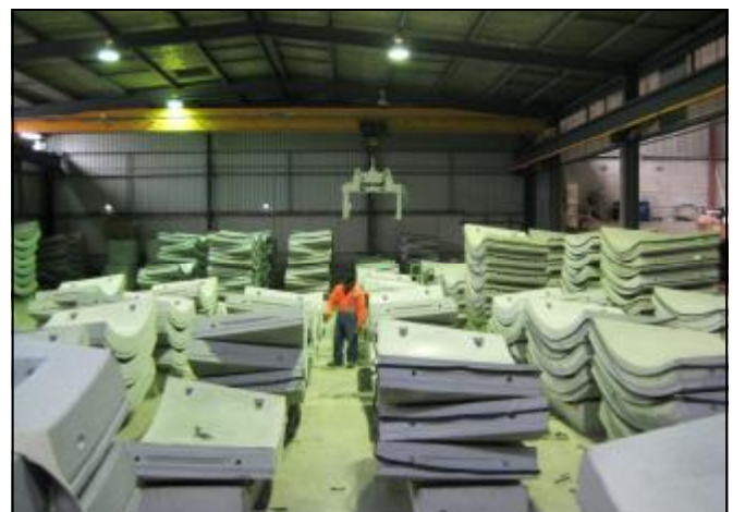
Completed segments ready for delivery
