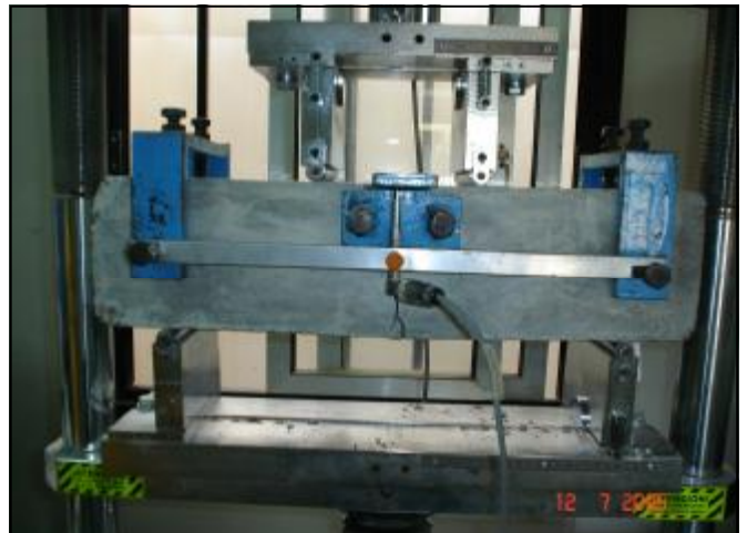
Testing in progress to reduce rebar content
