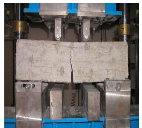
Flexural tests on concrete beams
